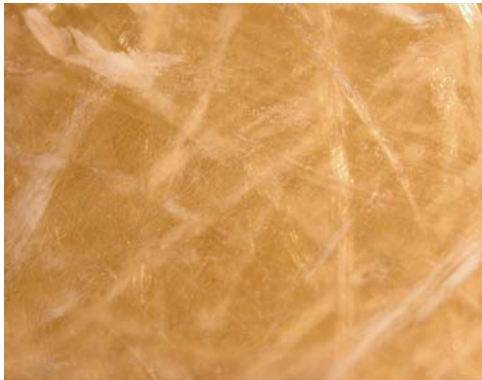
Surface of a GRP laminate showing prominent fibre magnified 32x
