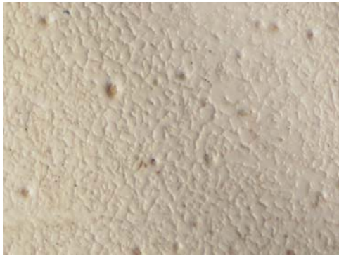
Surface of GRP laminate magnified 32x showing pinholes in the pigmented surface
